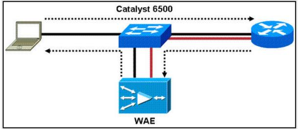
The WAE appliances are connected to Cisco Catalyst 6500 Series Switches and use WCCPv2 for traffic interception. The customer wants to minimize the latency added by interception. The customer also wants to know if Layer 2 redirection, rather than GRE tunnels, will improve performance.
