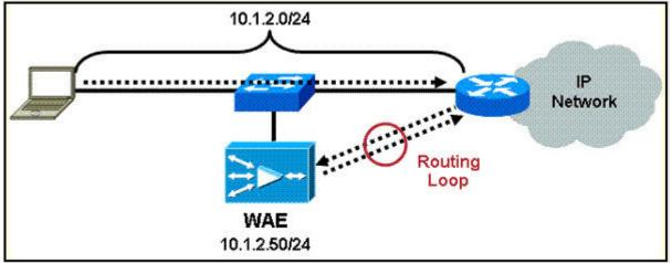
The servers that are being optimized are on subnet 10.1.2.0/24, and the WAE has been configured with the IP address 10.1.2.50. The customer has observed that routing loops have resulted from this configuration.
